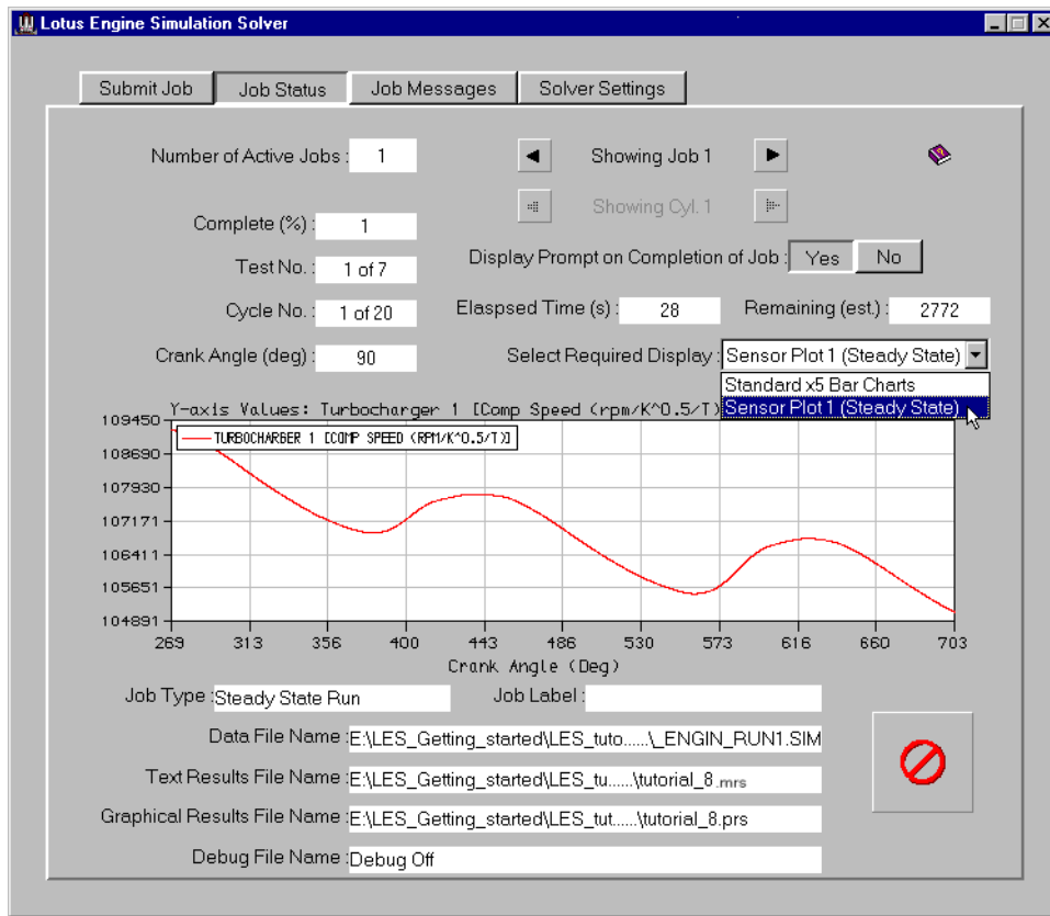
Figure 9.12. Runtime monitoring of turbocharger speed using sensor plot.
